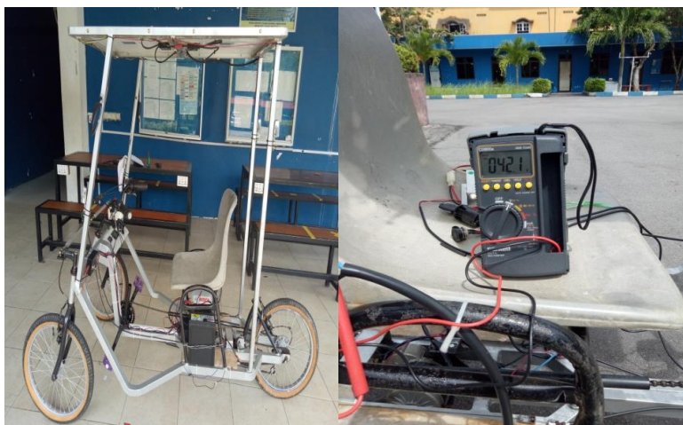
Figure 5. The Measurement of Voltage and Current from Solar Panel
